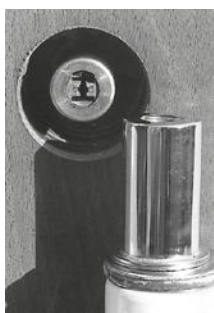
After the arriving the hard plate, get out the protector and unscrew the cylinder. Time used: 7 minutes.
